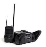
Equipped with cameras and adjustable tracks. This robot is mainly used for remote observation.
