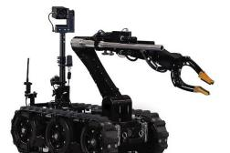
This robot is equipped with an arm that can move objects or even open doors. There are multiple cameras and microphones/speakers for remote communication. The tracks allow it to reach areas that are tougher to reach for smaller robotics.
