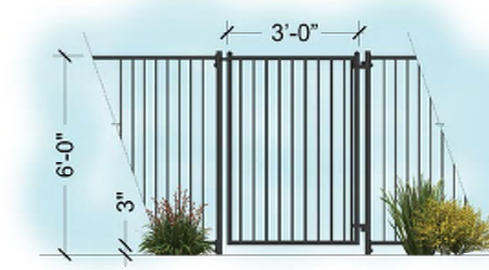
GATE: W-08 6'-0" TALL 3'-0" WIDE TUBULAR STEEL ACCESS GATE
