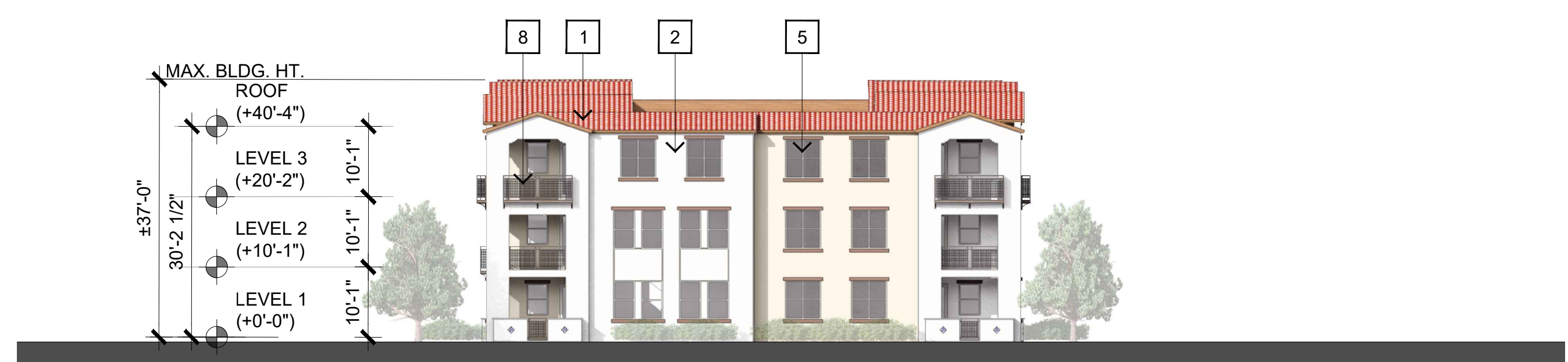
SOUTH ELEVATION (BLDG 3) BLDG 4 (MIRRORED AND SIMILAR)
