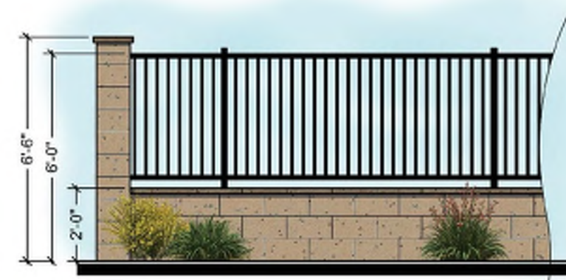
WALL: W-07 6'-0" TALL TUBULAR STEEL FENCE W/ RETAINING WALL
