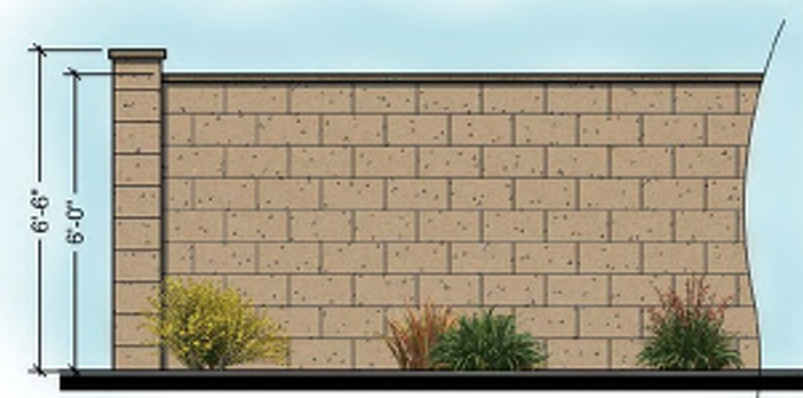
WALL: W-01 PILASTER: W-02 6'-0" TALL SPLIT-FACE BLOCK WALL W/ PRECISION BLOCK CAP
