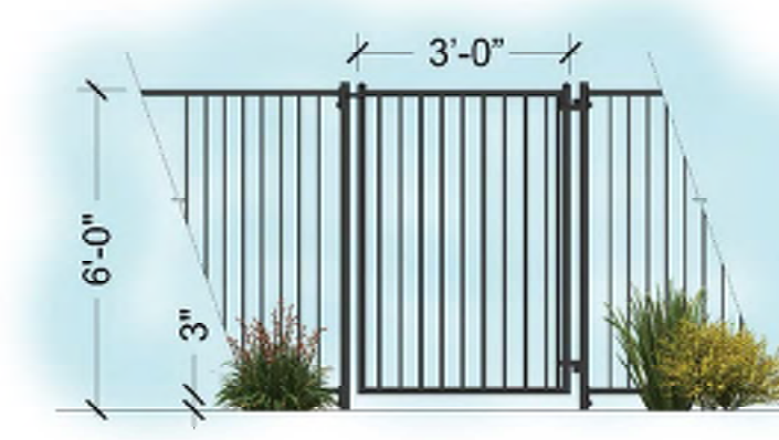
GATE: W-08 6'-0" TALL 3'-0" WIDE TUBULAR STEEL ACCESS GATE
