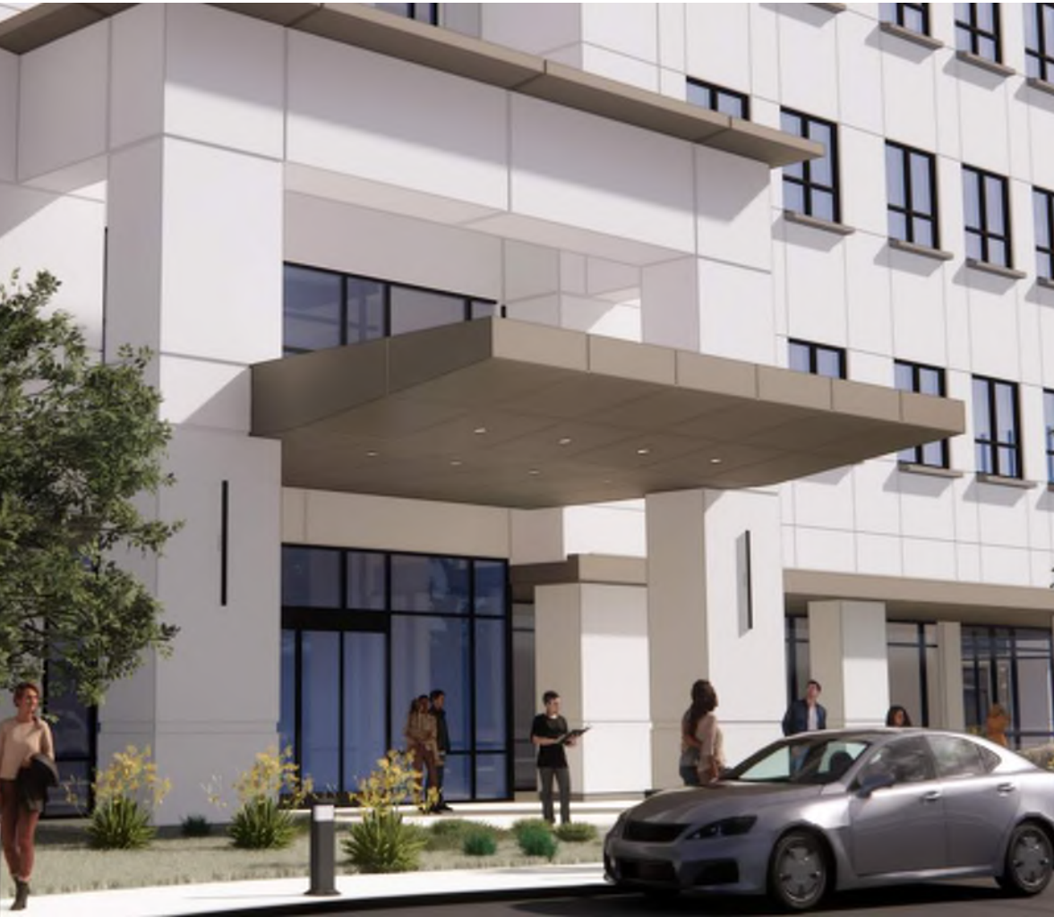
Aluminum composite metal (ACM) panels at building arrival canopies and pedestrian arcade Anodic Satin Mica
