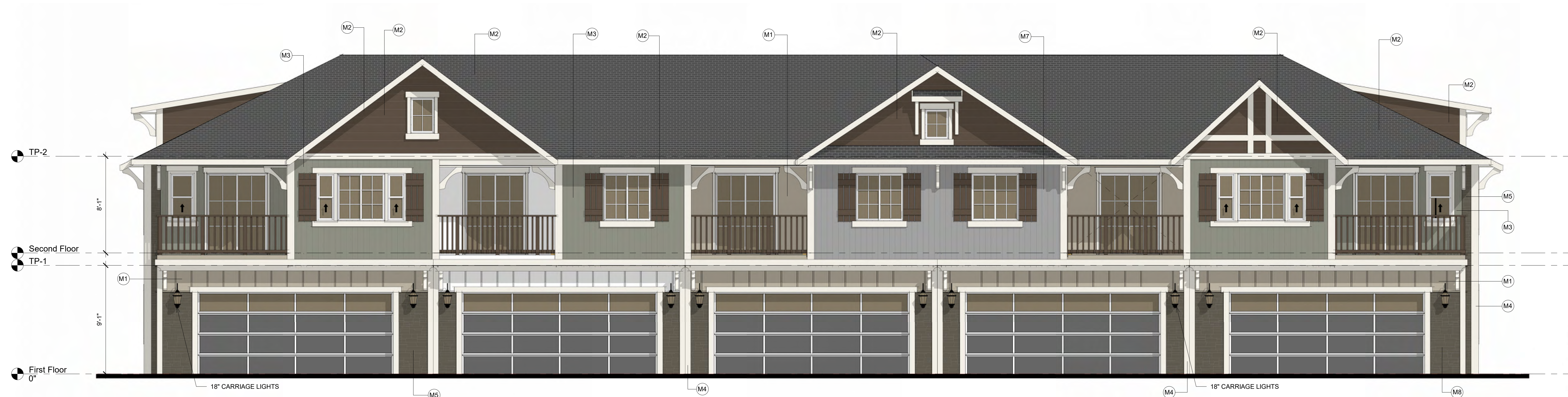
Rear Elevation - Type "B" (5 unit) 1/4" = 1'-0"
