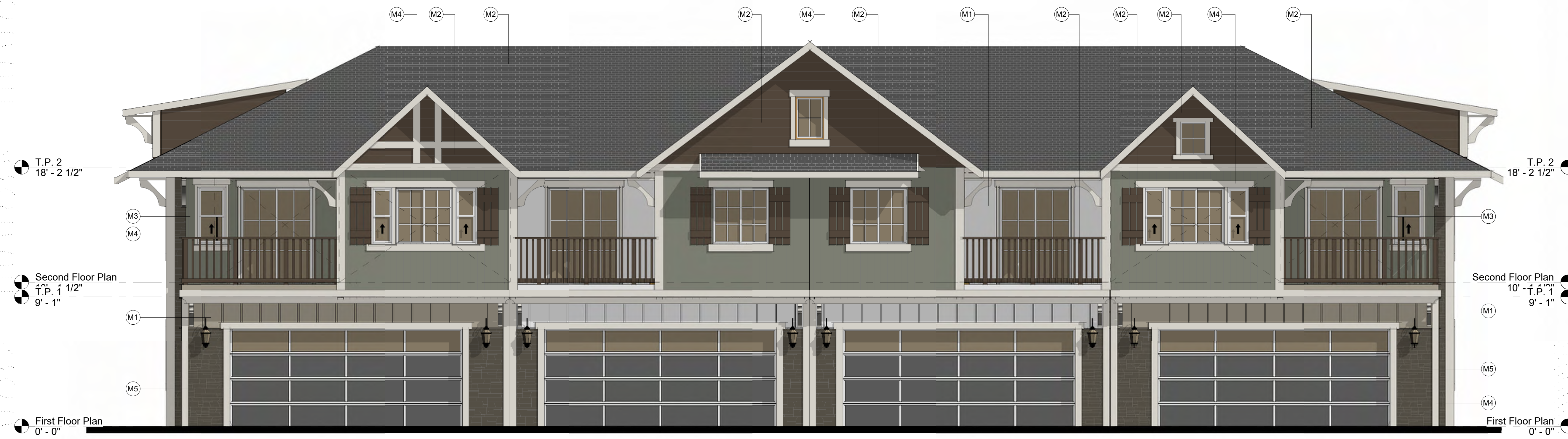
Rear Elevation - Type "B" (4 unit) 1/4" = 1'-0"
